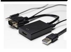
aura VGA to HDMI Adaptor Analogue to Digital. This VGA with 3.5mm audio to HDMI convertor enables the connection of a HDMI cable, screen or projector to an VGA output connector from a PC or laptop, comes with 10cm Fly lead, supports video and audio.
