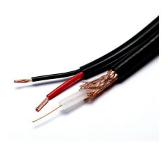
Aura RG59 Shotgun is a 75ohm coaxial cable and 0.5mm or 0.75mm red/black Power cable for CCTV systems. Cable features 0.58mm Dia copper clad steel inner conductor, Solid PE insulation, copper clad aluminium braid and PVC or LSZH outer sheath both meeting Eca standard. Also features red and black insulated stranded copper power conductors in overall PVC/LSZH outer sheath.
