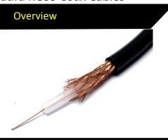
Aura RG59 is a 750hm coaxial cable with 0.58mm Dia copper clad steel inner conductor, Solid PE insulation, copper clad aluminium braid and PVC or LSZH outer sheath both meeting Eca standard.
