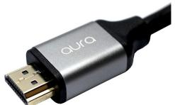
These high quality 4K 60Hz HDMI cables are made using 26 to 28 AWG copper cores with similar shielding ensuring strong signal abilities and good protection against outside interference. Connectors are robustly constructed with gold plated contacts. Insulation of the cables is a TPE outer sheath providing greater flexibility. Meets HDMI Standard V2.0
