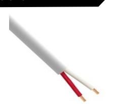
Aura OFC Speaker Cable made from 16AWG OFC Copper with 2 Core 41x0.2mm strands in a LSZH Eca White sheath 100M in plastic free packaging. Also available as Cca Fire rating in 2.5mm and 4.0mm core size's on 100m drums.
