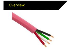
Aura OFC Speaker Cable made from 16AWG OFC Copper with 4 Core 41x0.2mm strands in a LSZH Eca Pink sheath 100M in plastic free
